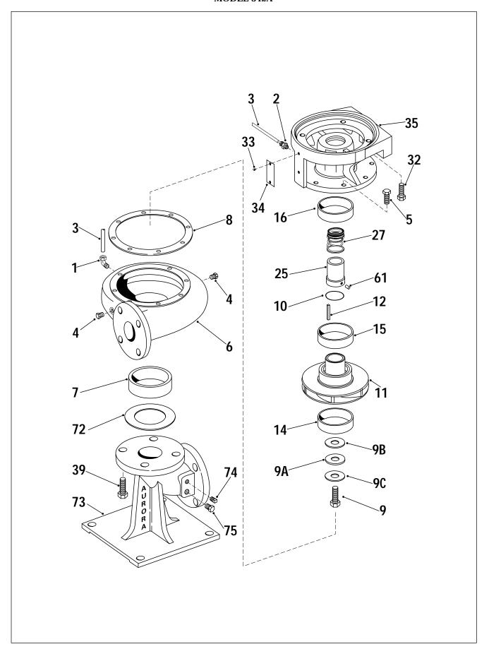
Figure 3. Model 342A Exploded View
